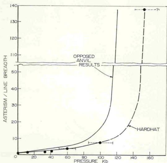
Fig. 11. Asterism/Line Breadth ratios from opposed-anvil pressurization experiments compared with data from material from known pressure zones of the Hardhat and Sedan nuclear explosions (Short, 1966). The horizontal dashed lines give the estimated pressure error (N. M. Short). The point plotted at 150 kbars is for the Sedan event for which the upper limit of pressure is not known. The other plotted points are for the Hardhat samples.
