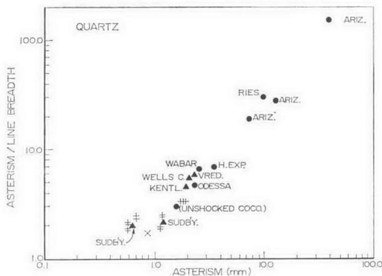
Fig. 6. Trend of the Asterism/Line Breadth ratio as a function of Asterism for quartz grains taken from various sources. The abbreviations refer to samples listed in Table 1. The symbols †, +, and × represent quartz grains from metamorphic, volcanic, and single crystal specimens respectively. Samples from shatter cones are indicated by triangles.
